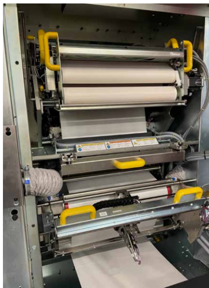
LED-UV curing station with chill roll on CX500t press
