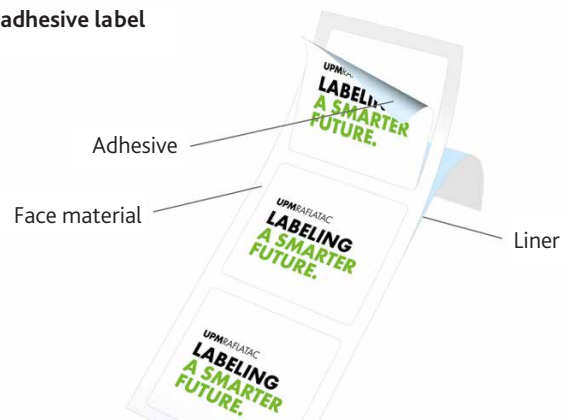
Composition of self-adhesive roll (courtesy UPM Raftatac)
