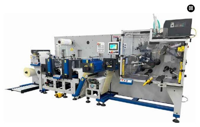
shipments and lost profits. The new Labelmaster delivers digital finishing, including rapid setup and on-the-fly changeovers and cutting without the need for tooling and die inventory.
